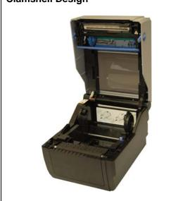
The cover stays open resting on the safety latch. The safety latch locks the printer top cover open when top cover is raised more than 45° upwards.
